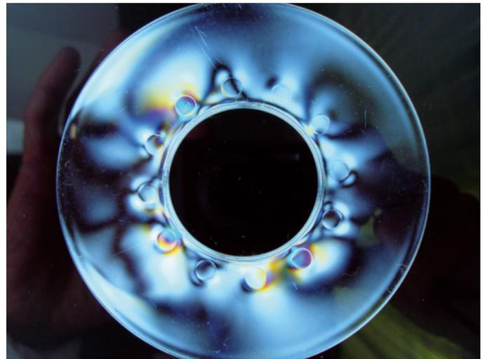
**Birefringence stress tests showing effect on moulded in stress of using small gates (Figure 2, left) and large gates (Figure 3, right)**
