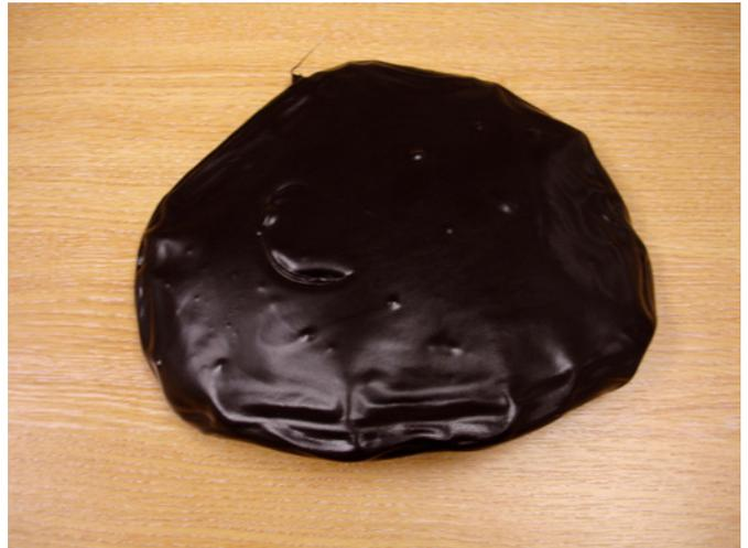
**Melt obtained using fast screw rotation and low screw back pressure (left) compared to the much more homogenous melt obtained using an optimised screw recovery and screw back pressure setting and a more controlled screw recovery time (right)**
